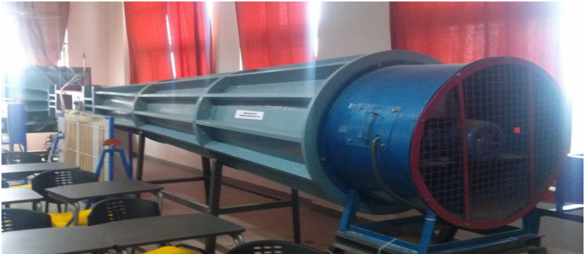
Figure Low speed wind tunnel equipped with 6 HP fan (with a test section of 1m x 0.3m x 0.3m and an overall length of 14 m)
