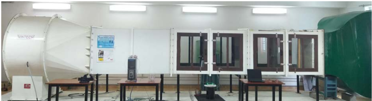
Figure Low speed wind tunnel equipped with 30 HP Axial fan (with a test section of 6 m x 1m x 1m and an overall length of 12 m)
